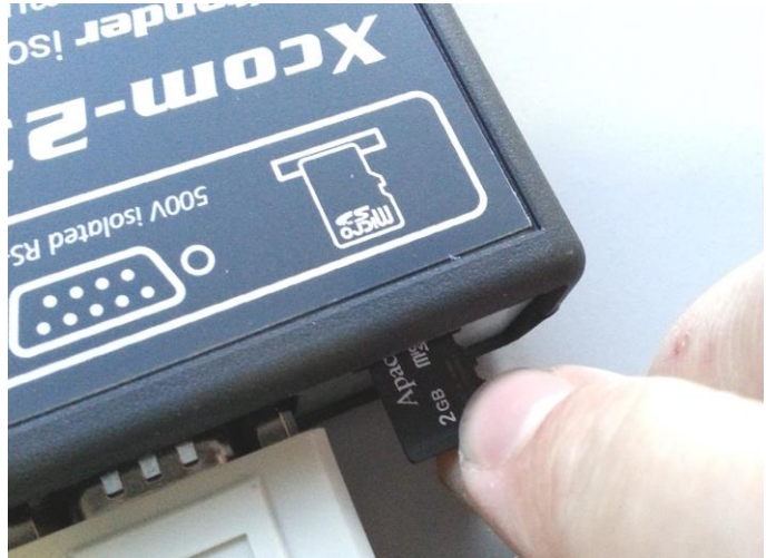
Figure 8 : Inserting the SD card
