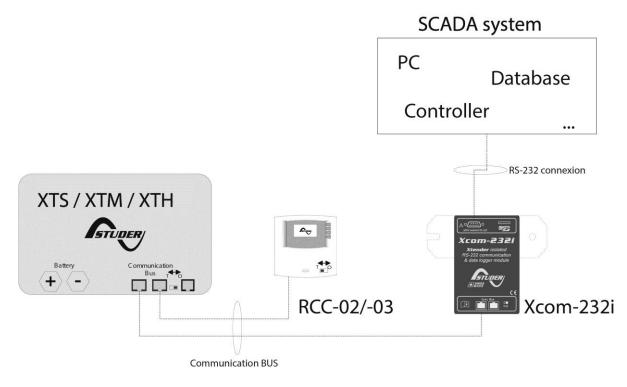
Figure 3.1: Connection schematics of the Xcom-232i (Example 1)
