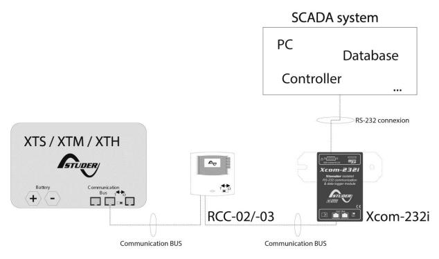
Figure 3.2: Connection schematics of the Xcom-232i (Example 2)
