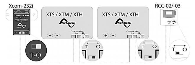
Figure 3.3: Online communication bus of an Xtender system
