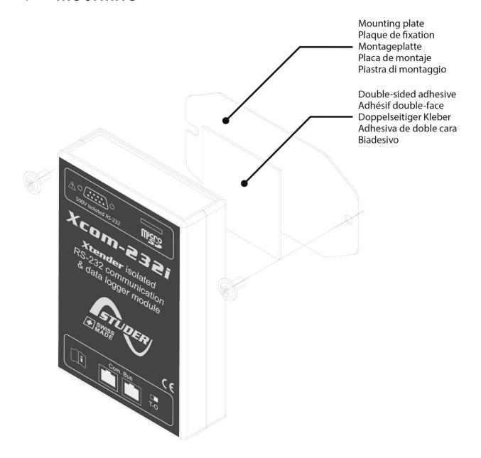
Figure 9: Mounting of the Xcom-232i
