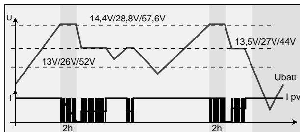
**NOTE: Since the solar charge controller integrated in the AJ is of PWM type, it is necessary to use 36 or 72 cell PV modules (12V or 24V respectively). All other types of PV modules require an MPPT charge controller (i.e VarioTrack or VarioString).**
